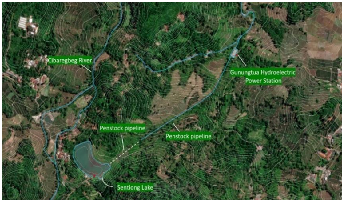
Figure 8. Water supply from Lake Sentiong to the Gunungtua Hydroelectric Power Station (Authors' Source).
