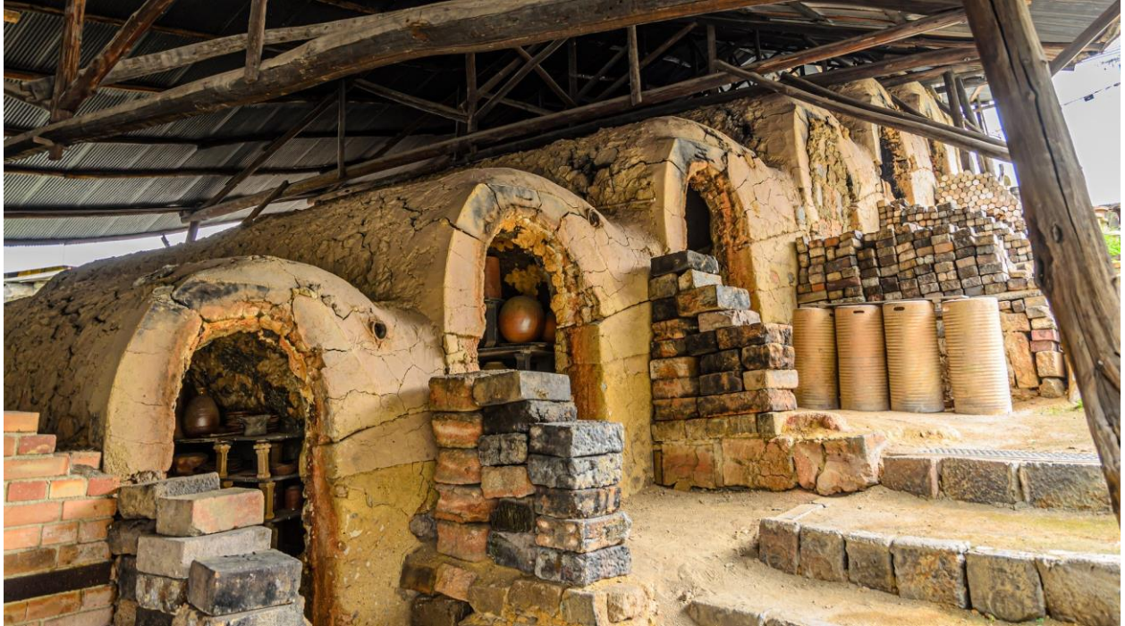
Figure 13. Le Sanpei Climbing Kiln's noborigama (Musubi Kiln, 2025).
