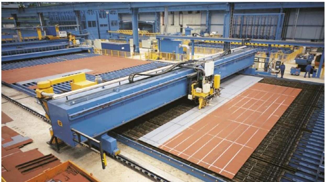
Figure 4. Laser arc hybrid welded steel panels and stiffeners used for fabrication of ships at Meyer-Werft GmbH (Acherjee, 2018b, p. 225).
