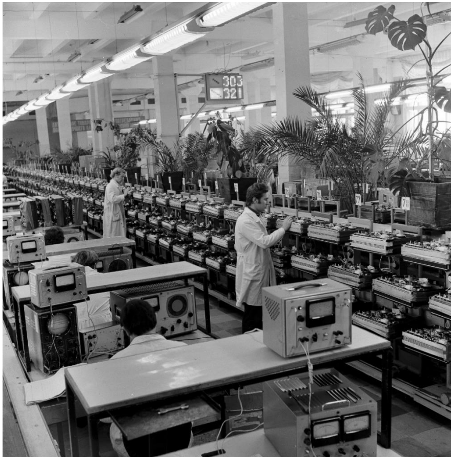
Figure 5. Adjustment and testing section of tape recorders at the Kyiv “Mayak” plant (Kyiv, 1980), illustrating the organization of calibration and quality control procedures in late socialist industrial production (Central State Audiovisual and Electronic Archive, n. d.).
