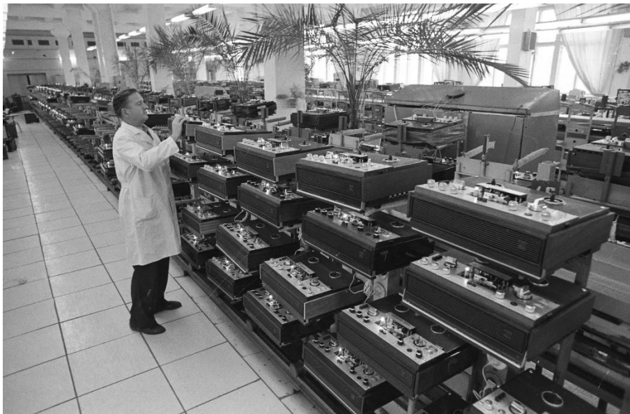
Figure 6. Tape recorder adjustment section at the Kyiv “Mayak” plant (Kyiv, October 24, 1979), illustrating calibration and fine-tuning procedures within the industrial production process (Central State Audiovisual and Electronic Archive, n. d.).
