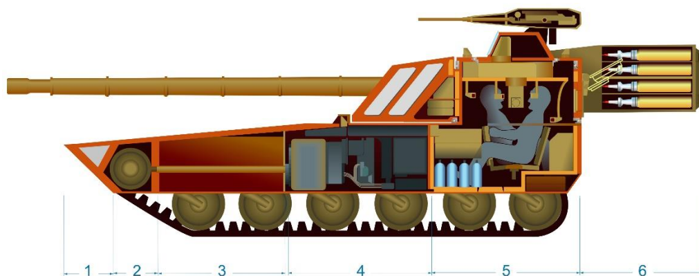
Figure 6. Variant of a non-traditional tank layout scheme with two guns. Author's reconstruction based on source (Apukhtin, Mazurenko, Morozov, & Nazarenko, 1980): 1 – hull armor, 2 – transmission compartment, 3 – fuel compartment, 4 – engine compartment, 5 – crew compartment, 6 – ammunition compartments with loading mechanism.
