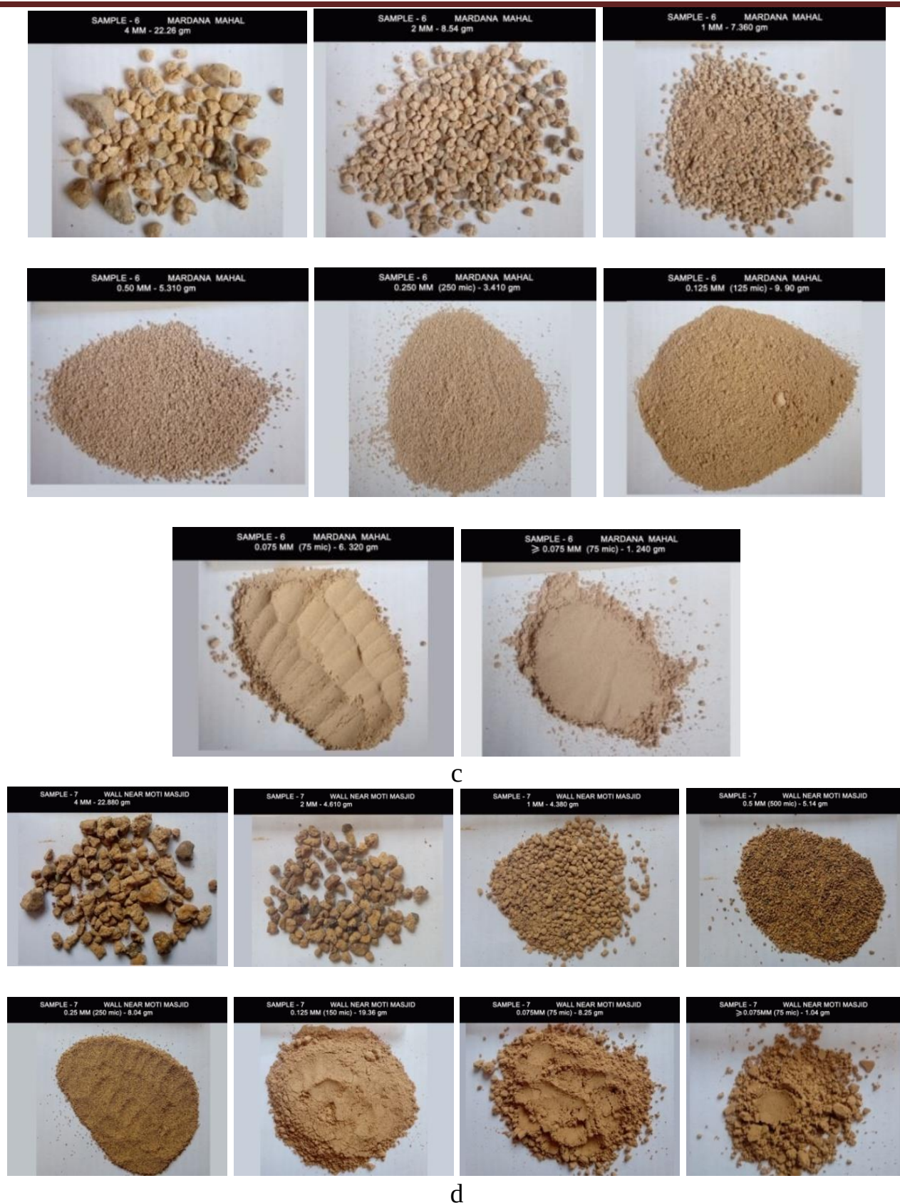
Figure 3. Acid insoluble aggregates in the plaster samples: a – No. 2; b – No. 5; c – No. 6; d – No. 7.
