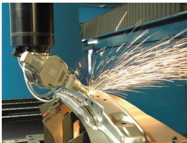
Figure 11. Three-dimensional laser cutting (3D fiber laser machine Rapido Prima Power).
