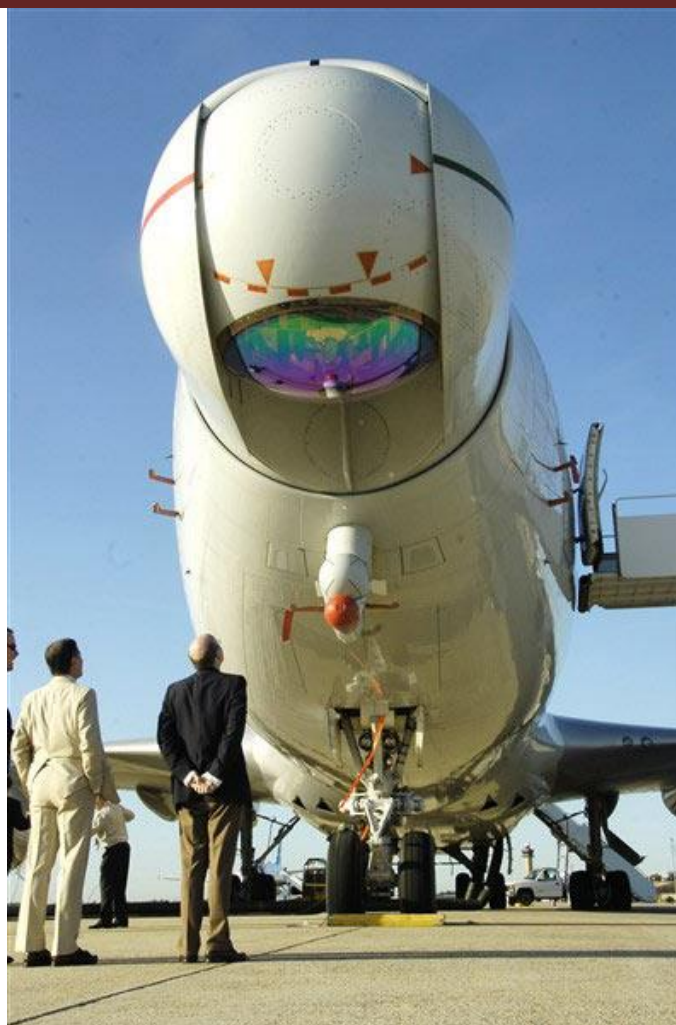
Figure 11. Boeing YAL-1 focusing unit (Rubial & Berges, 2012).
