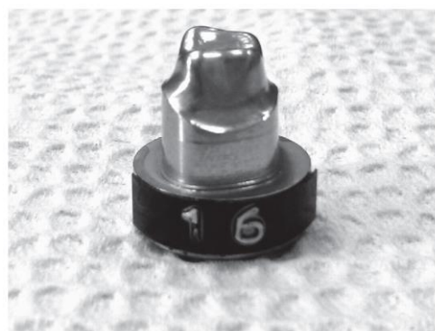
Figure 6. Dental prosthesis made using SLS technology (Kim et al., 2013).
