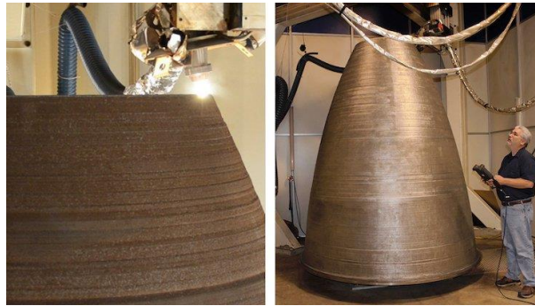
Figure 14. The manufacturing process and the finished nozzle of the 2 ton RS25 rocket unit (Davies, 2021).
