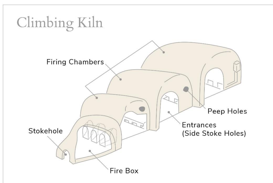
Figure 11. Climbing kiln scheme (Musubi Kiln, 2025).
