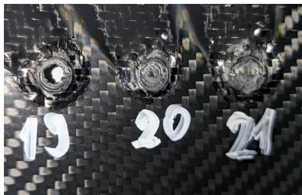
Figure 7. Example of the obtained results of the study of the effect of laser radiation on the carbon fiber-reinforced polymer plate (Authors' source).
