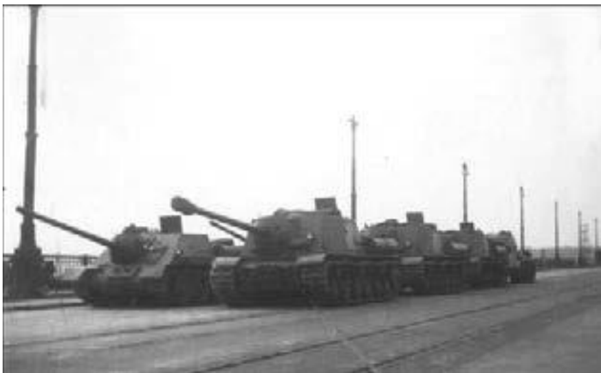
Figure 8. Testing of the bridge (Lobanov & Kyrian, 2013).
