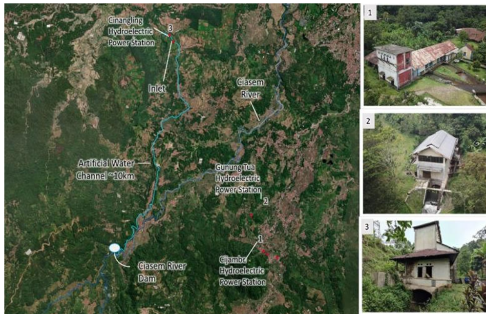
Figure 5. Water supply from the Ciasem River and the locations of three hydroelectric power stations: (1) Cijambe [6°37'53.24"S; 107°43'17.35"E], (2) Gunungtua [6°36'56.29"S; 107°43'19.93"E], (3) Cinangling [6°33'42.91"S; 107°41'8.38"E] (Authors' Source).
