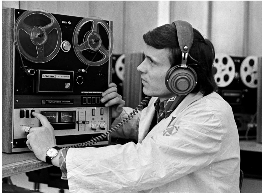
Figure 4. Quality inspection of a Mayak tape recorder at the Kyiv Scientific-Production Association “Mayak.” Technician Vitalii Solovei is shown calibrating a Mayak-001 tape recorder (Kyiv, March 17, 1976), illustrating factory-level testing and adjustment procedures in Soviet audio equipment production (Central State Audiovisual and Electronic Archive, n .d.).
