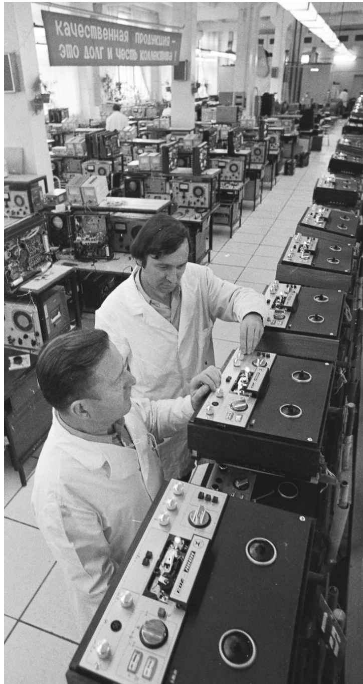
Figure 3. Radio equipment technicians at the Kyiv “Mayak” plant testing the operation of tape recorders on a testing bench (Kyiv, October 24, 1979), illustrating functional testing procedures within the industrial quality control process (Central State Audiovisual and Electronic Archive, n. d.).
